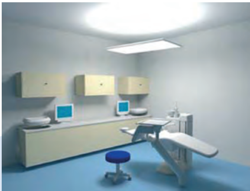
Light that has been sent back by the ceiling allows diffuses an harmonious lighting in the entire treatment room
